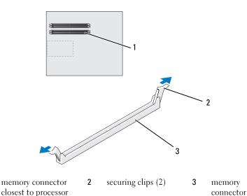
**4** Align the notch on the bottom of the module with the crossbar in the connector.
