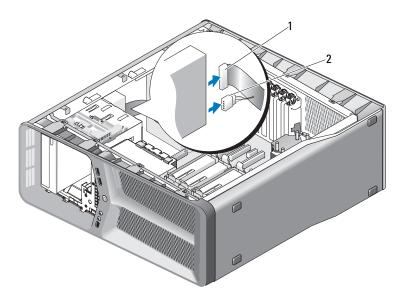
1 data cable 2 power cable **5** Slide the drive-release latch towards the base of the computer to release the shoulder screw, and then slide the CD/DVD drive out of the drive bay.
